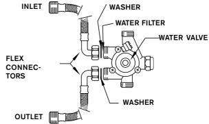
Fig. 6 - Water valve and water connectors, top view
