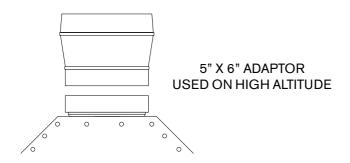
Fig. 3 - Vent Adaptor for High Altitude Installations
