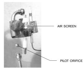
Fig. 9 - Pilot burner with air screen/ pilot orifice
