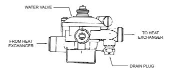
Fig. 0 - Water heater drain plug
