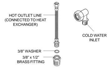
Fig. 3 - Water connections
