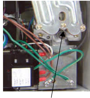
Manifold pressure tap.
